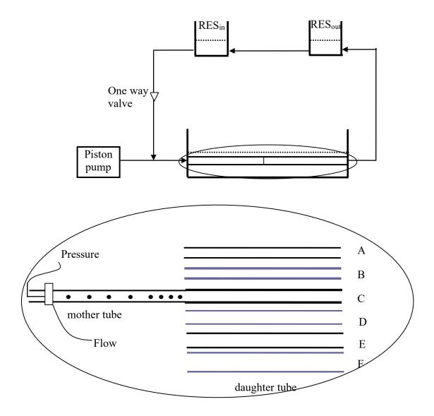
**Figure 1:** A schematic diagram of the experimental setup.  $RES_{inlet}$  and  $RES_{outlet}$  are the inlet and outlet reservoirs which provided the initial pressure to the system, and kept the tube free of air. Pressure and flow were measured using transducer tipped catheters, and ultrasonic
